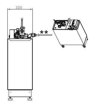
THREE-PHASE MOTOR: From 2.7 up to 13 CV (2 / 9.5 kW) 230 V-400 V-415 V; (50/60 HZ)
