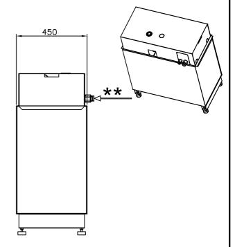
THREE-PHASE MOTOR: 230 V-400 V-415 V; (50/60 HZ) From 6 up to 25 CV (4.5 / 18.5 kW)
