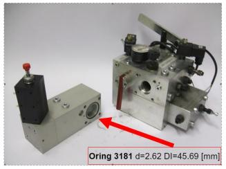
**Note:** with the spare part (code 659017G02) containing the various replacement O-ring, there are 2 O-rings type 4187 (d = 3.53 mm Di = 47.22 mm) which are not to be used.
